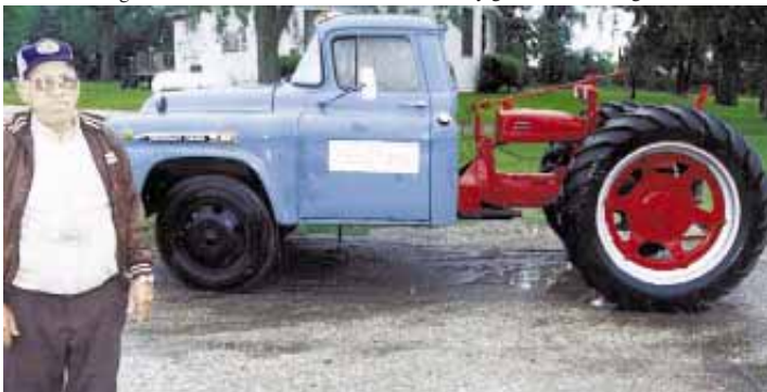
Leahy’s “Trucktor” consists of the back half of a 1940’s Farmall H tractor and the front half of a 1960’s Chevrolet 2-ton truck.
