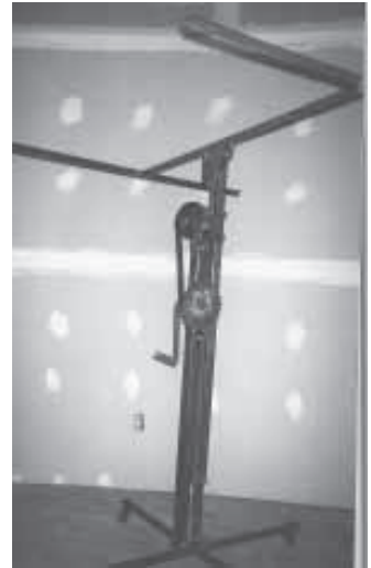
"It lets me do ceilings and walls by myself, taking my time to do the job right," says Dyck about his home-built drywall jack.
