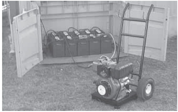
Portable charger can be used to charge a large bank of lead acid batteries.
