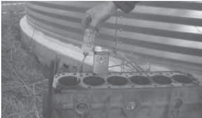
Applicator dispenses chemical around cylinder wall. It can also be squirted in through spark plug or nozzle openings.
