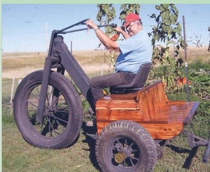
Warren Melcher used parts from an old riding mower to power this giant trike.
