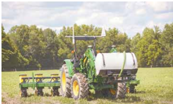
Kyler Laird has set up 4 robotic “tractobots” that drive themselves, including this Deere 6330 that’s used to plant corn.
