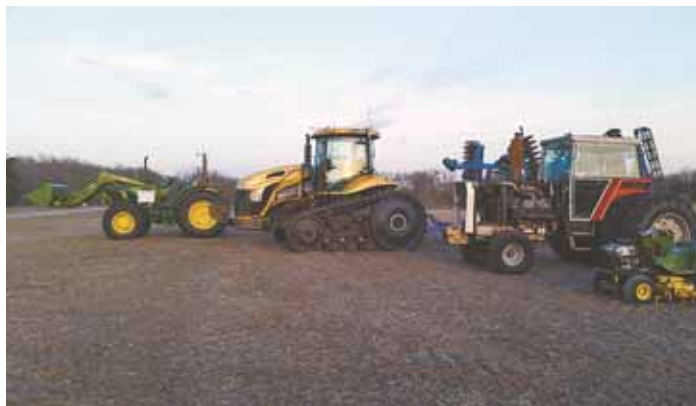
Laird also modified a Deere 420 garden tractor, an old Massey Ferguson to plant soybeans, and a Challenger for vertical tillage and pulling a grain cart.
