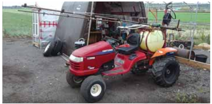
Garden tractor spray rig works great for fertilizing Reesor's 2-acre market vegetable operation. Extended frame on tractor makes room for tank and sprayer.
