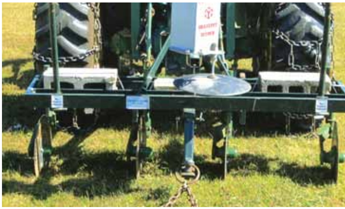
BRO pasture aerator uses 4 wavy coulters and a Shankpot Seeder for one-pass aeration and reseedling.
