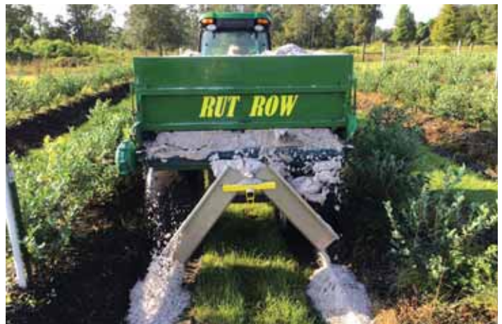
Sand hits a pair of aluminum deflectors on back of spreader and falls to either side, filling wheel ruts in blueberry field.
