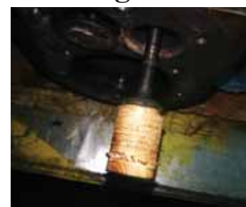
To grind down worn engine valves, Heron rotates the valve head using a 2-in. long wood plug from a hole saw.
