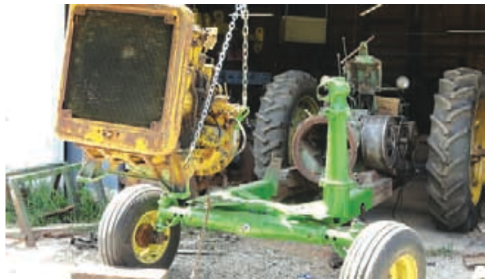
The first challenge Fenske faced was building a transfer case or right angle gearbox between the in-line Cat engine and the crossways Deere drive.
